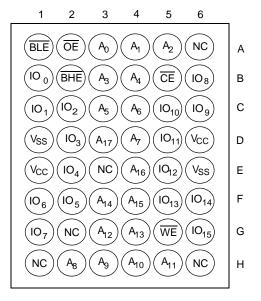
Figure 3. 48-Ball VFBGA (Pinout 2) [3, 4]
